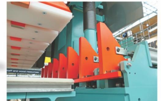
Top and bottom layer is clamped in place by last pressure element and moveable stopper.
