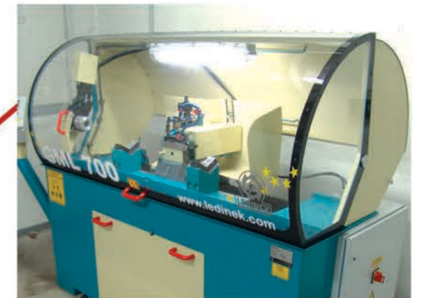
Fully enclosed cover with large windows. Schutzhaube mit großem Sichtfenster.
