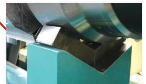
With adjustable support for different shaft lengths and bearing distances.
