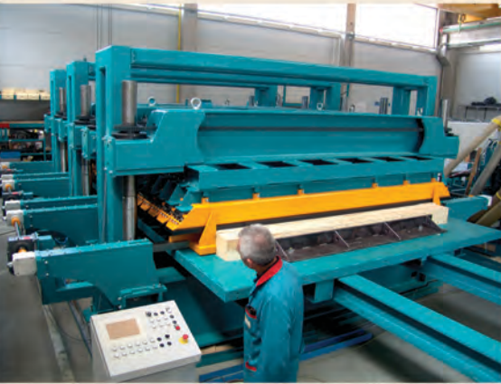
XPRESS Pressanlage für X-LAM (BSP, KLH, CLT, crossplan) Wandelemente. Pressing system for X-LAM (BSP, KLH, CLT, crossplan) wall elements.
