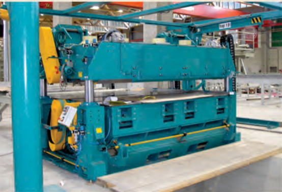
XPRESS Pressanlage für X-LAM (BSP, KLH, CLT, crossplan) Wandelemente. Pressing system for X-LAM (BSP, KLH, CLT, crossplan) wall elements.
