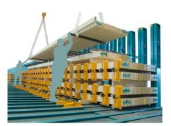
Fast glulam press with 4 press beds and motorized clamping
